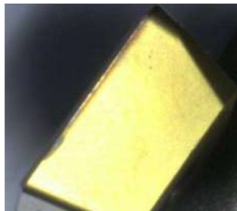
Fig. 6: Wear form of Central Insert [7].
