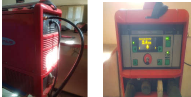
Figure 2. Pulsed TIG welding Machine setup
