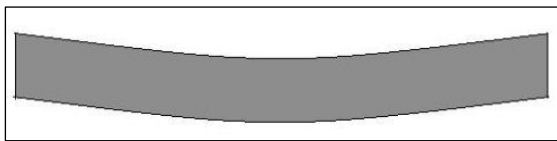
Fig. 7: Distorted Block after Welding.
