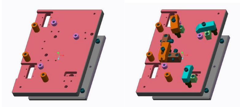
Fig 5 Base plate showing 3-2-1 location
