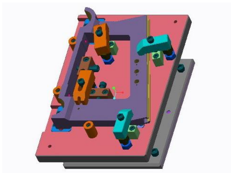
Figure 9 First setup of boring Fixture
