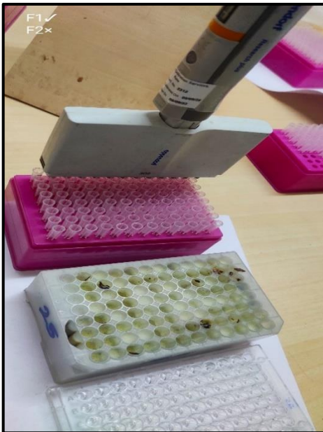
Figure-8: Sample addition (Multichannel Pipette)
