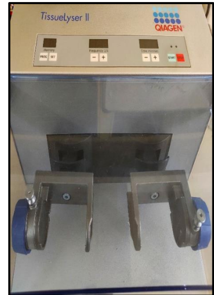
Figure-7: Crusher 17.5 Frequency 1/s
