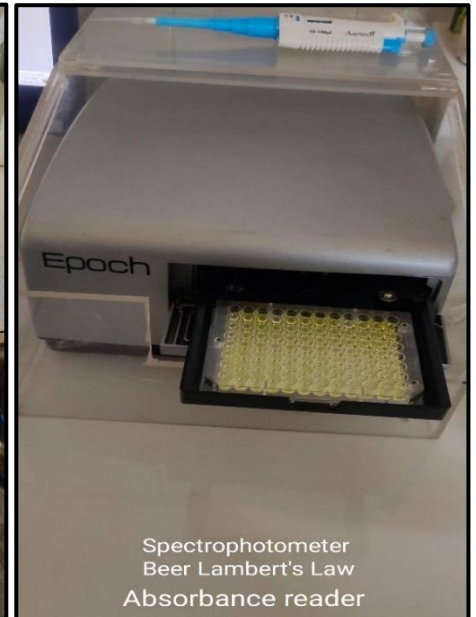
Figure-10: ELISA Microplate Reader with 450/620 nm Filter
