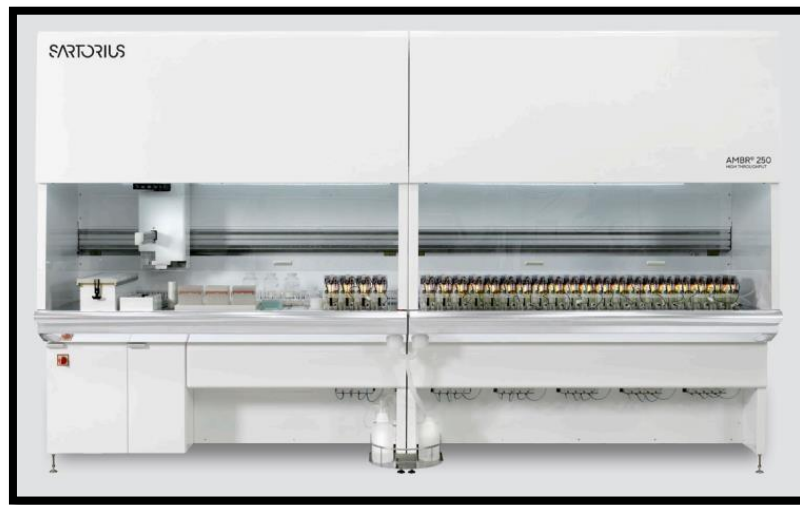
Fig 13: Ambr 250 high throughput system.
