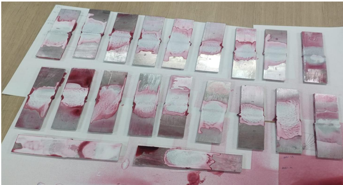
Fig 6.11 Application of developer on specimen [9]
