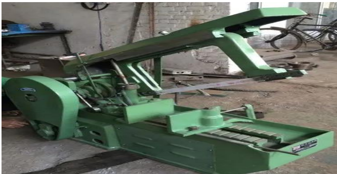
Fig 6.15 Preparing tensile test specimen using a Hacksaw cutting machine
