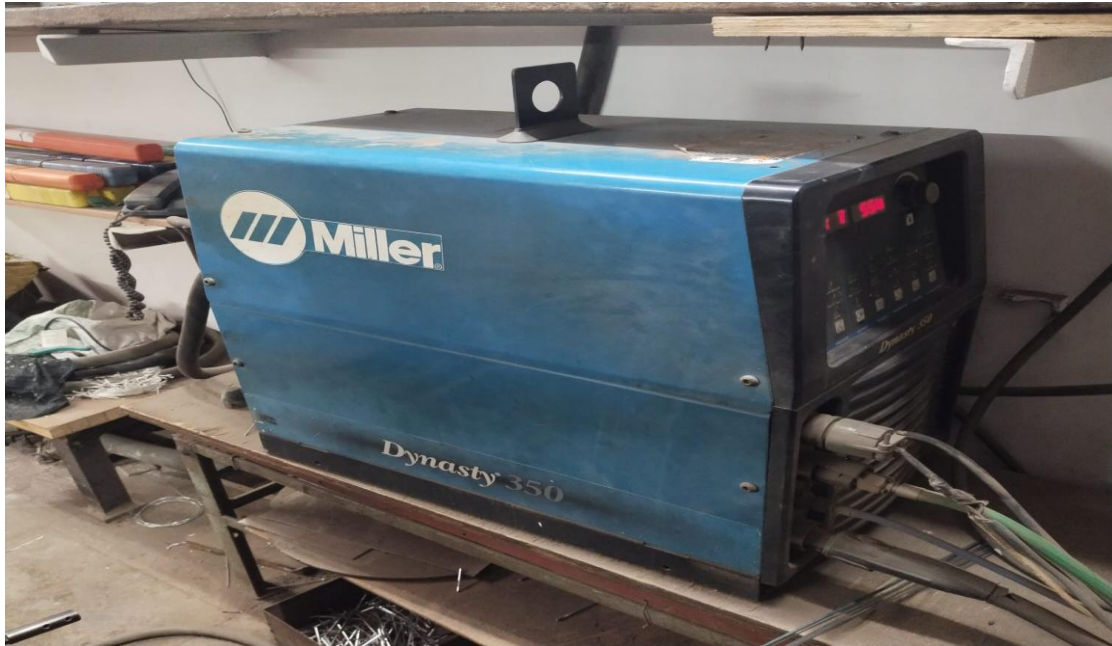
Fig 6.7 TIG welding machine setup
