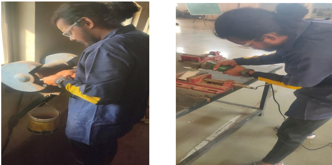
Fig6.5 edgepreparation on Hand Grinder
