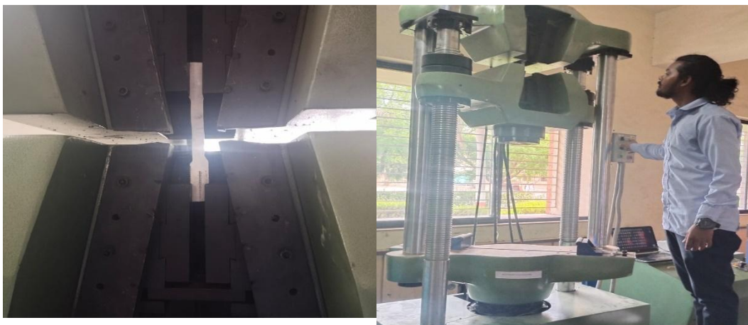
Fig 6.17 Tensile testing on UTM
