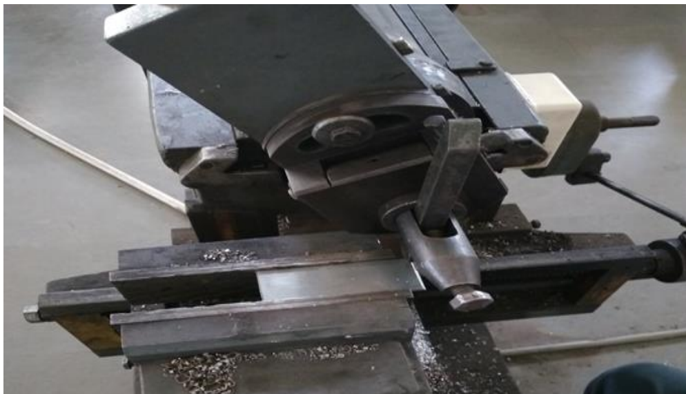
Fig 4.7- Weld edge preparation (WEP) on shaper machine
