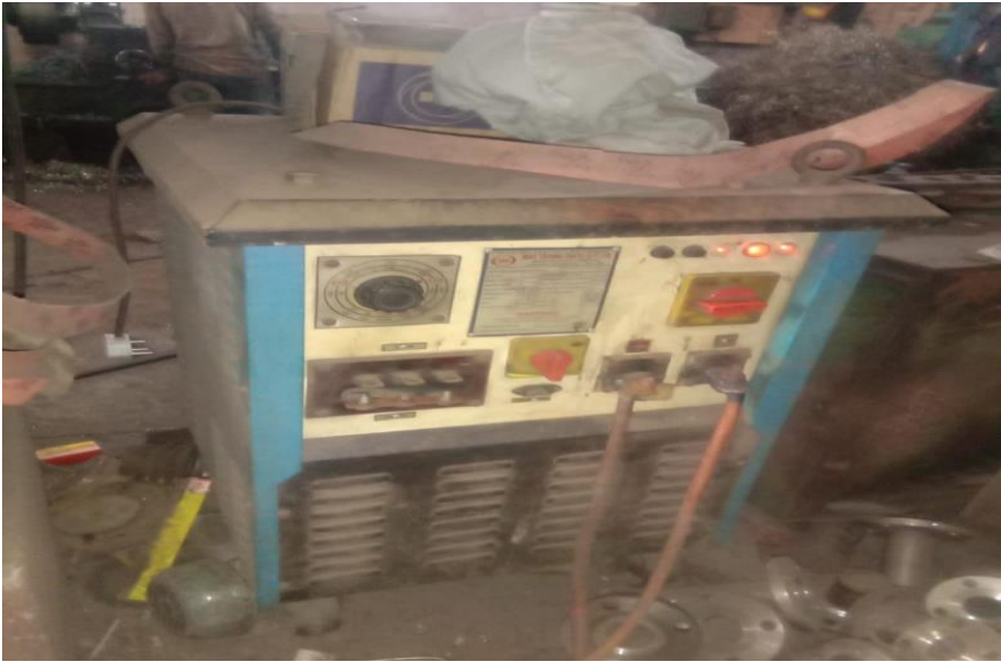
Fig 4.9 – TIG welding machine setup
