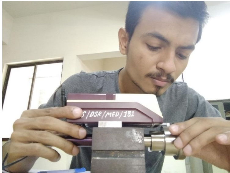
Figure 5.12: Checking and noticing Surface roughness value
