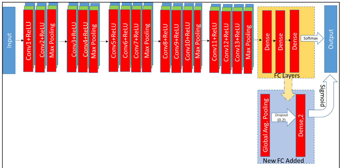
FIGURE 4.2: Architecture of VGG16, a CNN model. The FC layers of base model (highlighted by yellow rectangle). Modified VGG16 model (highlighted by blue rectangle)
