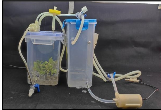
Figure: 3.2 Temporary immersion system designed in Plant Biotechnology Laboratory to study in vitro growth of Musa acuminata
