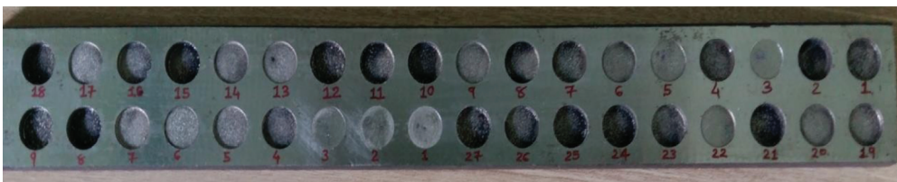
Figure 3. Impressions of the tool on work surface after machining.
