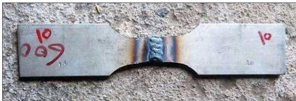
Fig. 2: Specimen SS-304 with TIG Welding [4].
