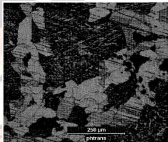
Mixed bainitic-austenitic structure of 20 MnMoNi 55 after heating and cooling. Etched with 5 % HNO 3 solution
