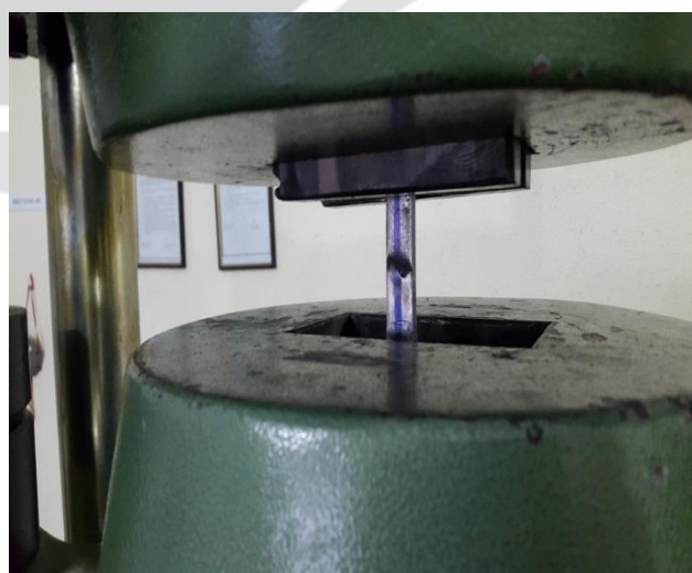
Fig -3 specimen under tensile test
