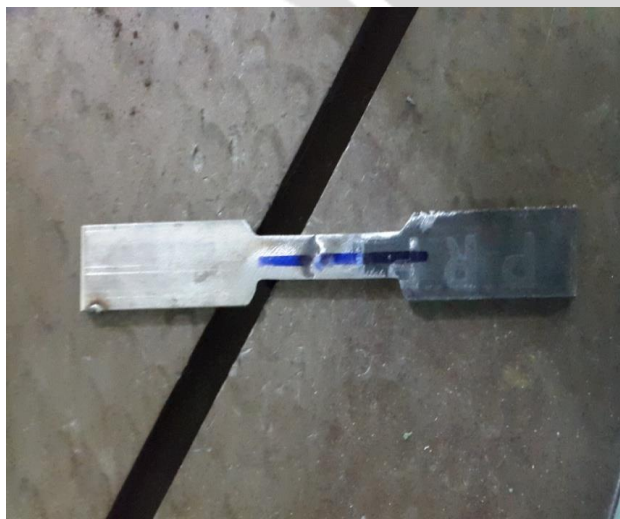
Fig -2 specimen for tensile test
