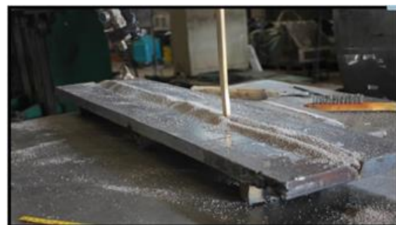
Fig. 1: Submerge Arc Welding at the Industry.
