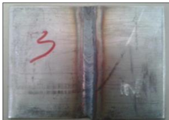
Fig. 1: Test Piece Welded Utilizing TIG Welding with 2.0 mm Root Hole.
