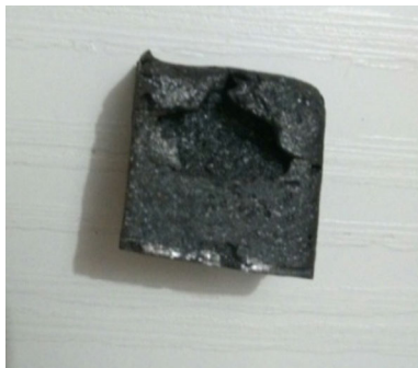
Figure 5. Sand inclusion defect.
