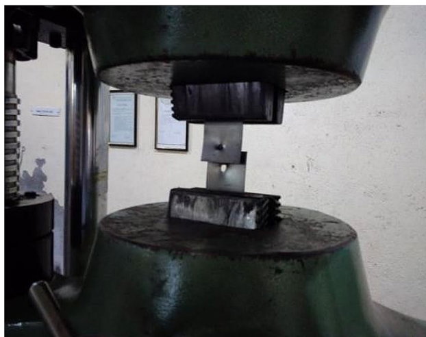
Fig. 4 Breaking load determination in Universal Testing Machine
