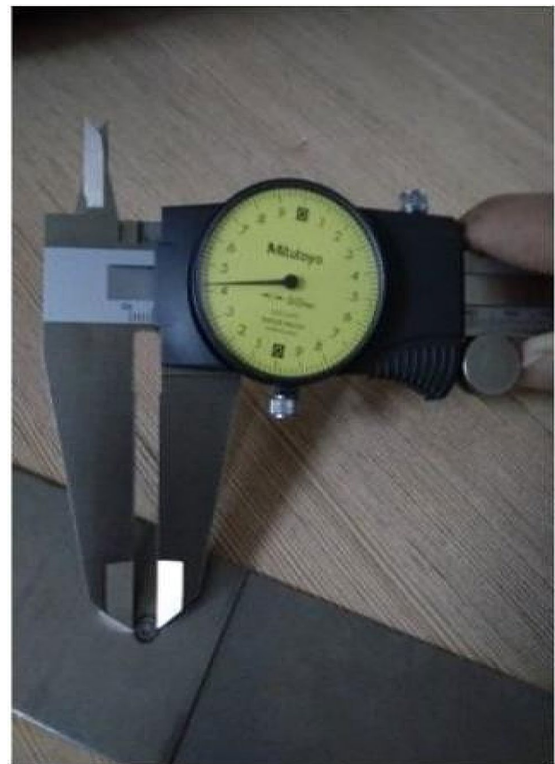
Fig. 8 Measurement of Nugget Diameter
