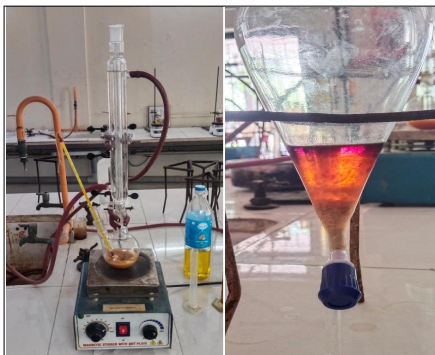
Figure.7 Biodiesel reaction process and gravitational Separation of biodiesel, glycerol & other unreacted components
