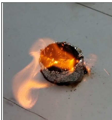
Figure.11 Flame Test of Biodiesel
